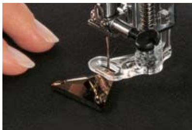
Sew-on Stones Switch off the lower feed and adjust the stitch width to the product.
