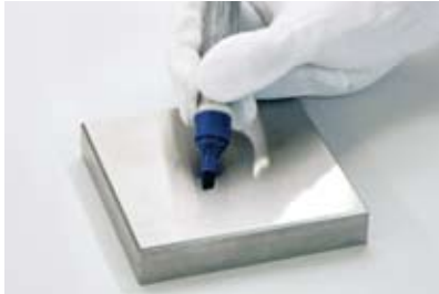
1 The surfaces to be glued must be properly pre-treated to achieve a sufficient surface tension. This can be tested via a test pen.
