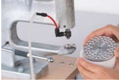
1 Place the revolving magazine in the setting frame.
