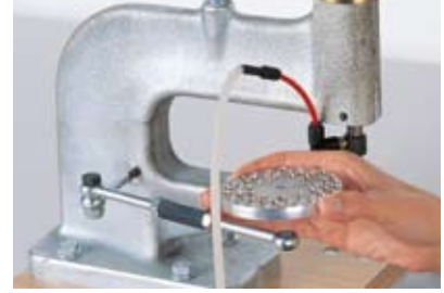
3 Place the magazine with the Rivets into the holder.
