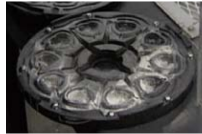
3 Channels are cut in this rubber plate for the casting process.
