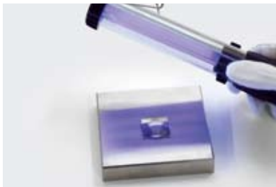
4 Cure the glue for a few seconds using a UV light (following the manufacturer's instructions), and remove any excess glue using a cleaning agent. The curing process can then be continued, according to the manufacturer's instructions.
