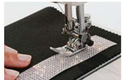
Crystaltex Bandings Sew between the rows of stones.
