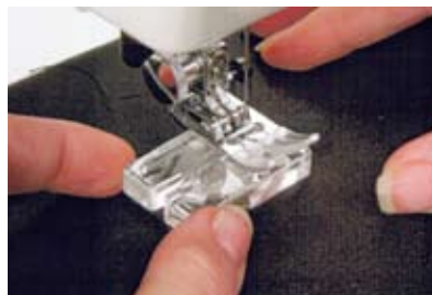
Place the aid for the Sew-on Stone 3265 underneath the foot and choose a button sewing program or a zigzag stitch. The lower feed must be turned off.
