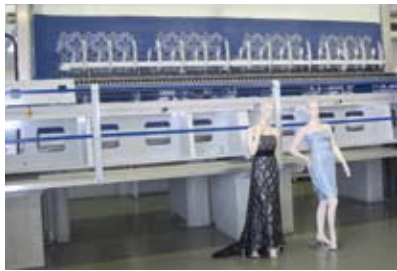
4 Embroidery is carried out automatically using the Lässer Challenge Crystal Stone system.
