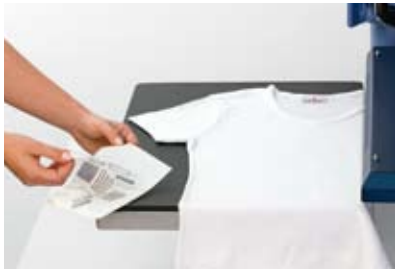
1 Peel off the white protective film*.
