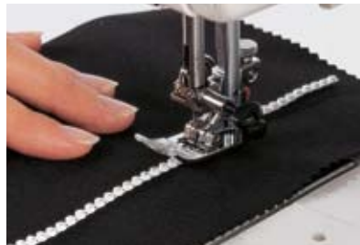
Basic Bandings (single row) Make sure that the Basic Banding runs parallel to the foot.
