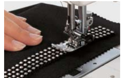
Basic Bandings (multi row) Stitch the banding between the first and second rows of crystals and if necessary strengthen the corners with a zigzag stitch.
