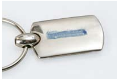
2 If the ink remains visible for 2 seconds, the surface is suitable for gluing.
