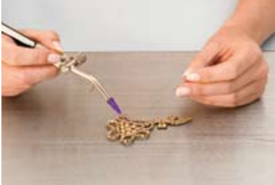
1 Soldering the original model
