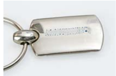
3 If the ink disappears or forms bubbles, the surface is not suitable for gluing. In this case, the pre-treatment cleaning methods should be checked.
