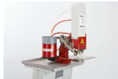
Some SWAROVSKI ELEMENTS can be applied using fully automatic attaching machines (e.g. Rose Pins). In this process, the feed on the machine must be adjusted to the element being processed.
