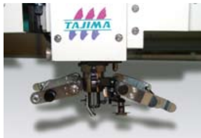
The lock stitch head is ideal for applying Crystal Yarn and single-row Plastic Trimmings.
