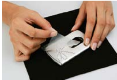
5 After the glue has hardened, remove the transparent film (taking into account the technical data of the glue).
