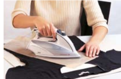
3 A Teflon® underlay protects the soleplate of the iron from any glue residue.
