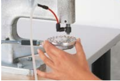
4 The Rivets are taken up by means of the vacuum.
