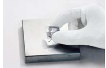
3 Press down on the crystal, until the glue completely covers the gluing area.
