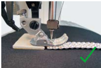
The foot lies flat due to the height compensator .
