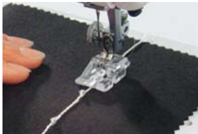
Crystal Yarn Make sure that the Crystal Yarn runs parallel to the foot.
