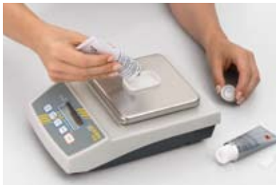
1 Weigh out the two glue components at a ratio of 1 : 1.
