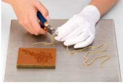
1 Cut the Cupchain to the required length.
